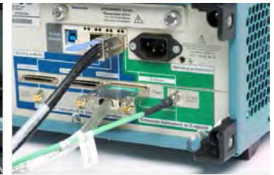
UltraSync connection on instrument with Extension role
