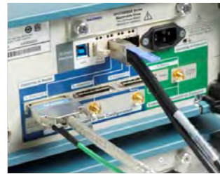
UltraSync connection on instrument with Master role
