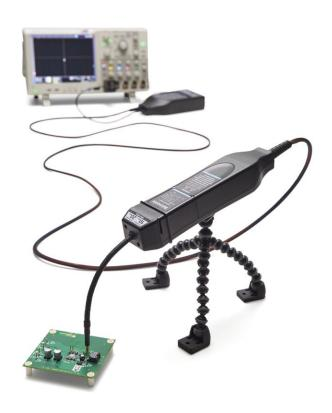
The Tektronix TIVM Series IsoVu™ Measurement System offers a galvanically isolated measurement solution for accurately resolving high bandwidth, differential signals up to ±50 Vpk in the presence of large common mode voltages with the best in class common mode rejection performance across its bandwidth.
