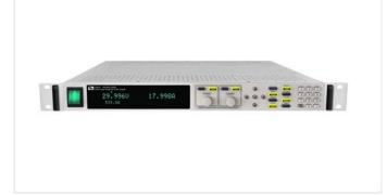
IT6500 series is a flexible range single output high power supply. With wide power ranges from 800 W to 6 kW, currents from 30 A to 240 A. Standard RS-232, USB, GPIB, RS-485 and LAN interfaces included on the rear panel provide flexibility for remote operation of the power supply. Its compact 1U (1.200W) to 4U (6 kW) size form factor makes it ideal for use in a standard 19-inch rack.
